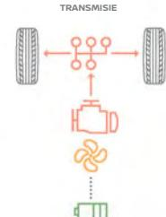
MOTOR CU ARDERE INTERNA GENERATOR BATERIE
